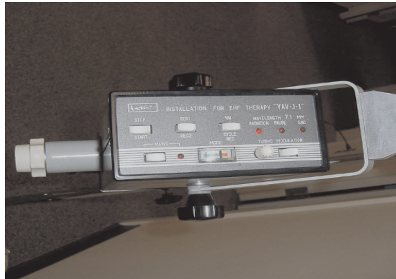
Figure 2. The YAV-1 MW Device. The instrument panel is shown on the left. Millimeter waves emerge from the rectangular horn seen within the circular white plastic applicator seen in the picture on the right.
